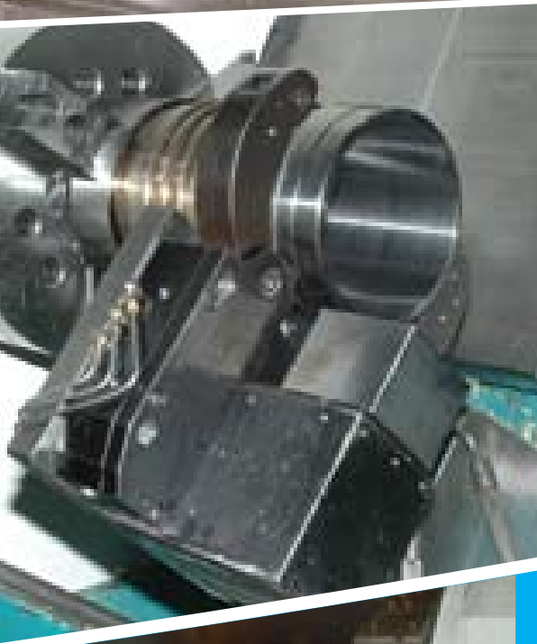
Steady Rest with Pneumatic Cylinder on Flat bed lathe, Travelling application - USA
